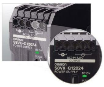
Simply click onto a standard DIN rail using one hand to mount in a flash. Effortless and time saving! In addition, the S8VK features a double set of DC output terminals (three for the negative terminal), which means you also spend less time and effort on wiring.
