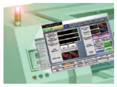
The machine designer can easily implement PLC troubleshooting, machine troubleshooting, settings for servo drives, temperature controllers, and other control components, status monitoring of connected devices, and uploading/downloading of parameters.
