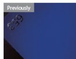
Low contrast makes the surface appear uniform.
