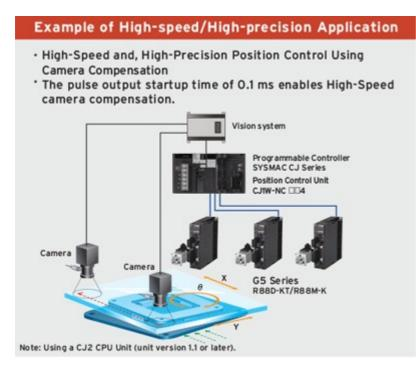
High-speed and High-precision Positioning
